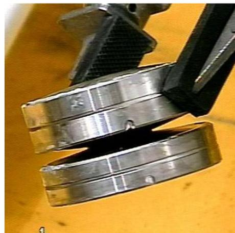
Fig. 2. Failed RbCl targets
