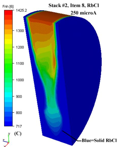
Fig. 3. Predicted temperature distribution in a RbCl target
